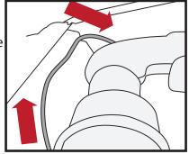
Step 6. Thread the supplied jam nut on to the end of the cable as far as you can. Apply RTV silicon sealant to the threads on the end of the cable. Install the supplied brass housing on to the cable and tighten down. Do not over tighten. Thread the brass fitting on by hand until it bottoms out on the cable. If the fitting is over tightened, the knob will begin to extend and you will need to back off the brass housing. Tighten the jam nut against the brass housing to secure the housing.
