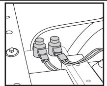
Engaged- Place the transfer case into four wheel drive. Press and hold the red push button on the control cable and pull the cable outward. The vehicle may have to roll slightly for the coupler to fully engage. Once the cable lock has fully engaged adjust the hold/release knob clockwise to secure the cable.
