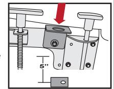
Step 2. Remove the jam nut and washer from the handle end of the cable. Start cable through the dash bracket. Place nut and washer over the end of the cable and continue the cable through the hole drilled in the firewall. Fasten cable loosely to the dash bracket with the jam nut and washer. Cut grommet on one side to form "C" and install grommet in the firewall to protect the cable from the sharp metal. Note: may want to put silicone lubricant on grommet for easier installation.
